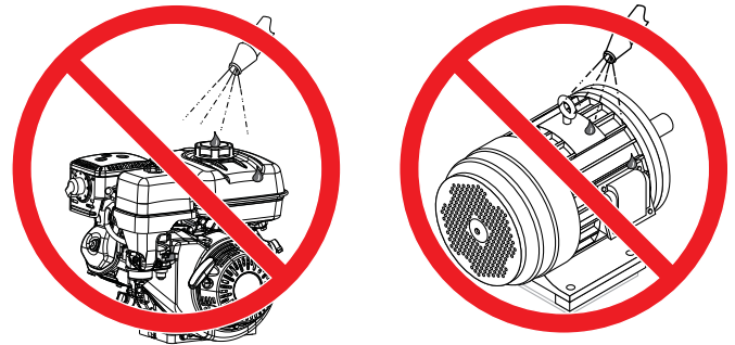
Figure 37. No Spraying of Water
