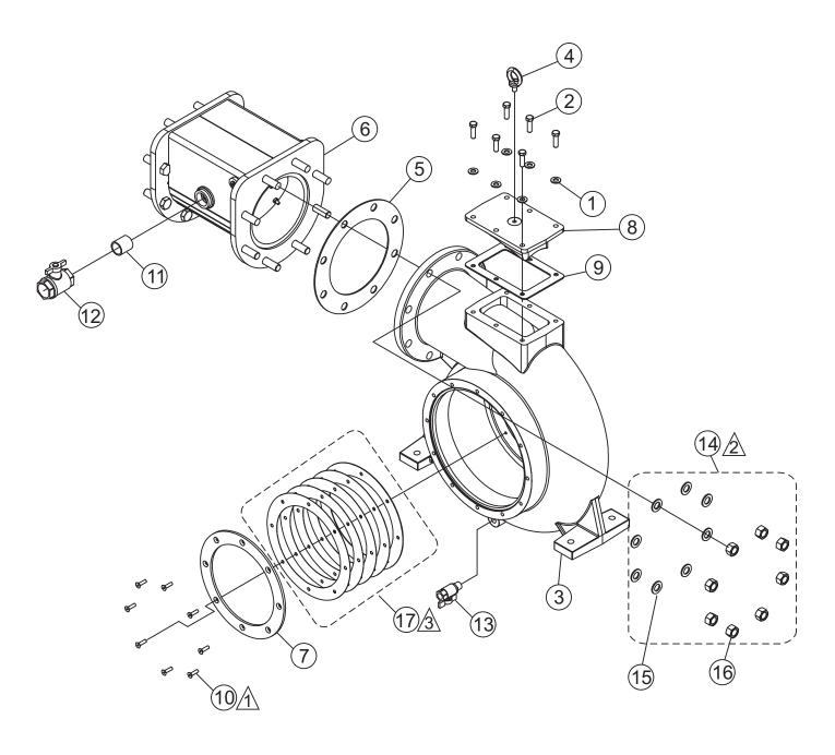
USE THREADLOCK: HIGH TEMP LOCTITE BLUE 246 OR EQUIVALENT. TORQUE TO 14 FT-LBS. (18.9 N-m).
