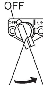
Figure 15. Engine ON/OFF Switch (OFF)
