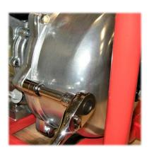
3. Remove the impeller by first rotating it counter clockwise until you feel the engine come to its compression stroke and stop. Using a hard plastic mallet, swiftly strike the end of one of the impeller veins hard CCW to break it free from the engine shaft and then turn it CCW by hand to remove it.
