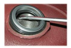
6. Pry and pull the worn mechanical seal half with rubber backing from the rear pump casing cover.
