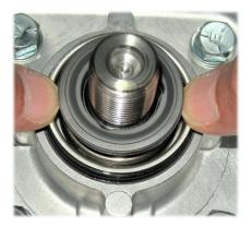
8. With the carbon surface facing outward/away from the impeller and covered by a clean strip of paper or cloth to avoid contaminating the seal surface, install the new mechanical seal half by pushing firmly and evenly on outer edge all around until fully seated into the back of impeller.
