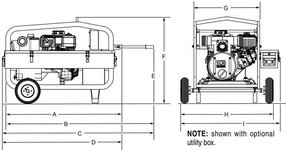
Figure 1. QP3Ti Dimensions
