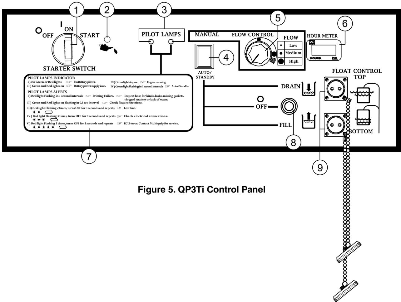
Figure 5. QP3Ti Control Panel
