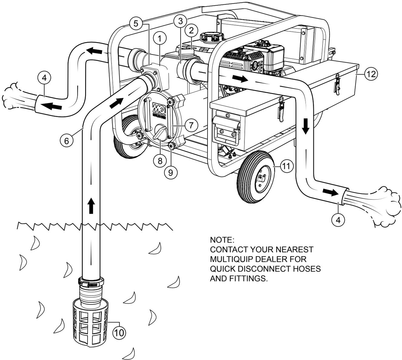
Figure 3. QP3Ti Key Components
