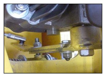
The two bolts shown in this picture are not to be tightened copletely. They are supposed to fit loose. The entire linkage assembly needs to be free flowing. If there is any binding on any of the shifting parts it will be very difficult to stop the creeping.
