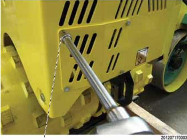
Figure 8. Front Cover Removal
