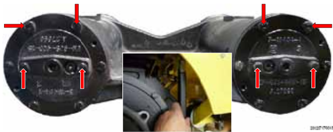
Figure 12. Screw Torque Adjustment (Rear Vibratory Unit)
