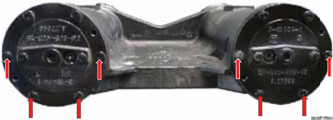
Figure 13. Screw Replacement (Rear Vibratory Unit)
