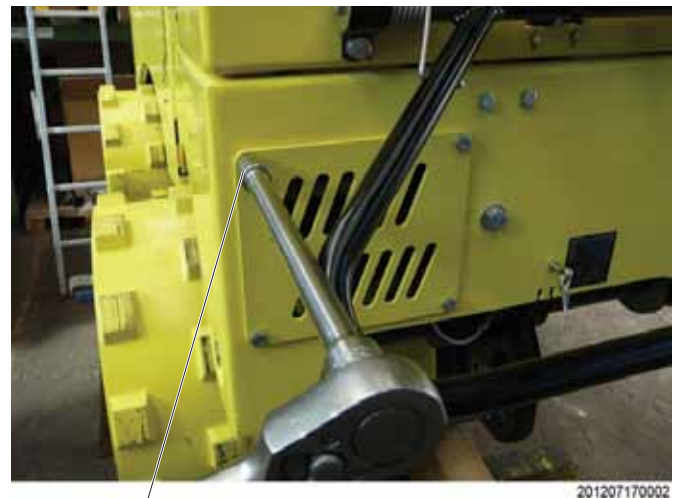
Figure 7. Rear Cover Removal
