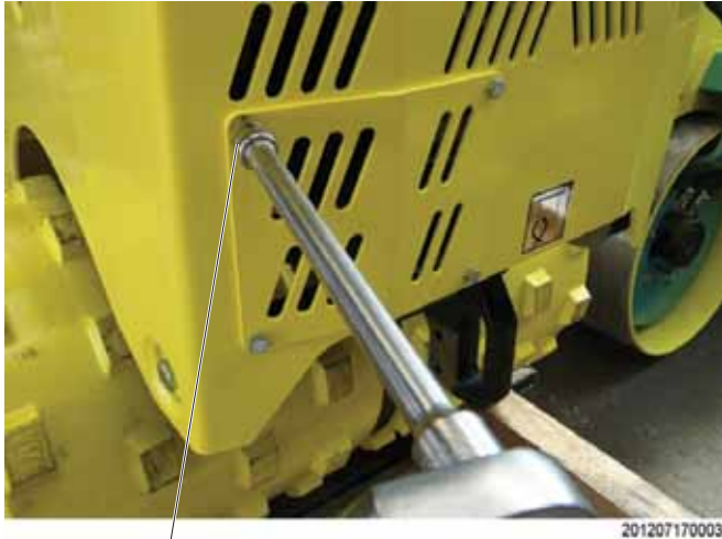
Figure 8. Front Cover Removal
