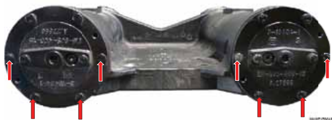
Figure 13. Screw Replacement (Rear Vibratory Unit)
