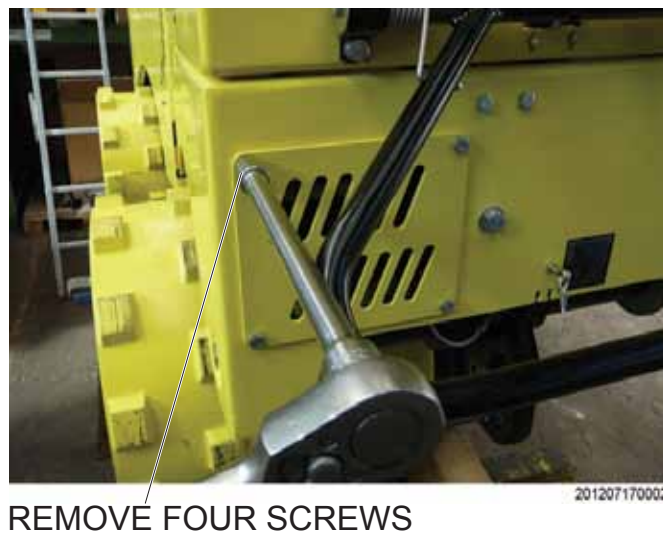
Figure 7. Rear Cover Removal
