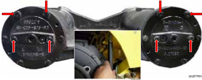
Figure 12. Screw Torque Adjustment (Rear Vibratory Unit)
