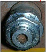
Note the location of the steering relief valve, located on the manifold block, left side from rear of roller. Remove the black cover to expose the adjustment screw.
