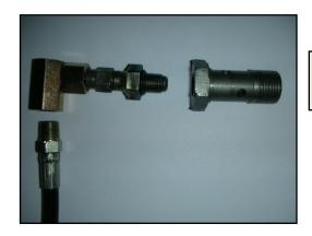
A custom banjo bolt fitting is needed to install gauge.
