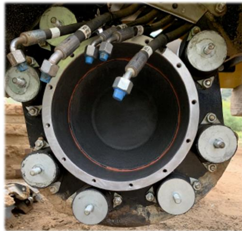
All exciter weights and bearings will come off with cover (heavy). Remove old grease from inside empty cavity.
