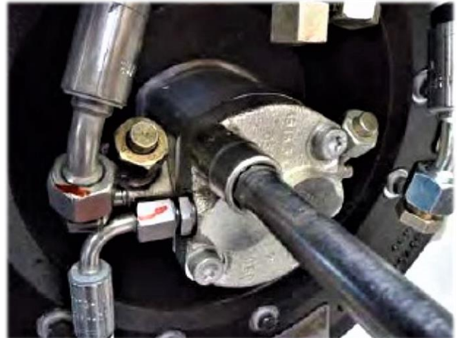
Two M10 bolts to mount the vibration motor (56 Nm)
