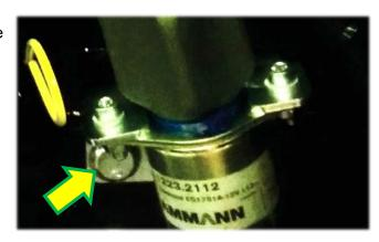
8) Push the throttle lever and the solenoid's lever so that the bolt holes align while maintaining a 2 mm air gap between the limit screw and fuel lever.
