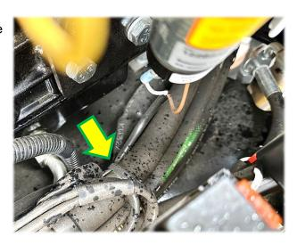
2) Remove the two 5mm screws that secure the solenoid to the engine mounting bracket.
