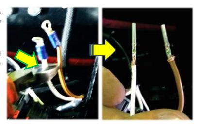
5) Insert wires with newly Installed Deutzch terminals ends into the Deutzch connector. When placing wires into the connector, make sure to match white to white.
