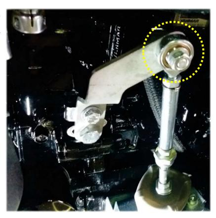
10) For use in setting the 2 mm control gap between the limit screw and fuel lever.
