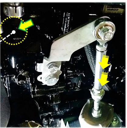
12) Position the solenoid in the maximum position and confirm that the gap is still set at (2 mm).
