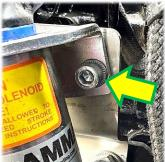
3) Disconnect the wires/terminals from the solenoid.
