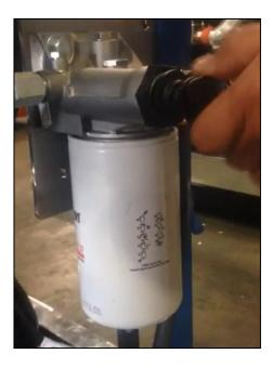
2. Pump the priming handle by pulling and pushing to pressurize the fuel system.
