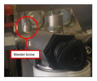
4. Repeat steps 2 and 3 until the air is removed from the fuel system.
