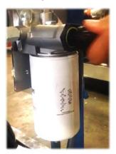
3. Crack open the bleeder screw on top of the fuel filter housing to release the air in the fuel system. Retighten the bleeder screw.
