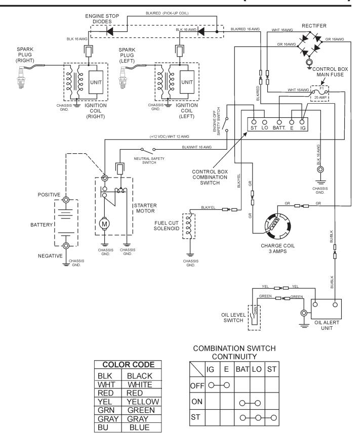
Figure 61. 20HP Honda Engine Wiring Diagram
