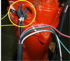
The (4) wires shown above, need to be capped and secured within the sleeve of the power harness.
