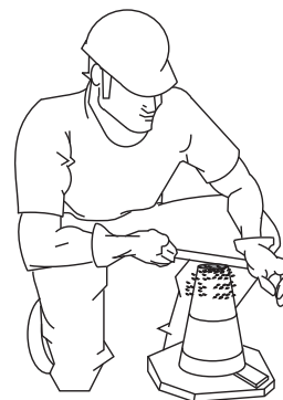
Figure 41-D. Slump Test (Removing Excess Concrete)
