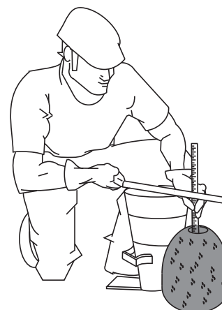
Figure 41-F. Slump Test (Measurement)
