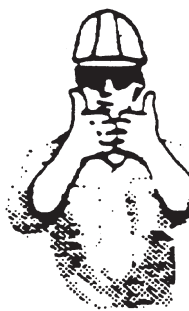
All Done Clean Up
