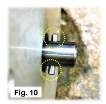
7) The gear has a keyway on one side, slide the gear onto the shaft so that the dowel is positioned in the keyway. Install a Starloc washer over the shaft to secure the gear in position. Ref. Fig. 11, 12 & 13
