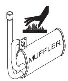
■ The engine section of this generators requires an adequate free flow of cooling air. **NEVER** operate the generator in any enclosed or narrow area where free flow of the air is restricted. If the air flow is restricted it will cause serious
