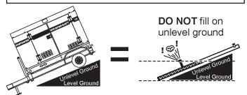
Figure 14. Only Fill on Level Ground
