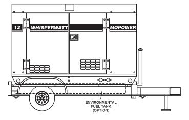
Figure 13. Internal Fuel Tank System
