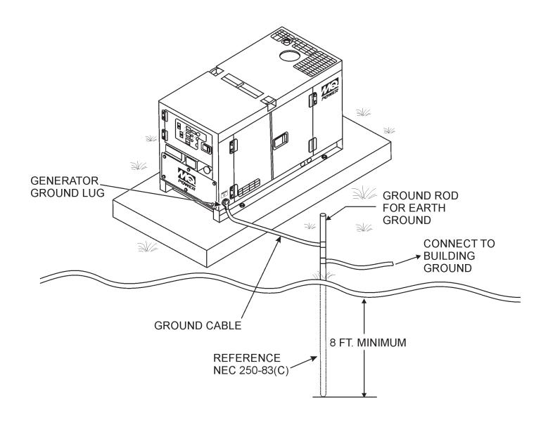
**Figure 2. Typical Generator Grounding Application**
