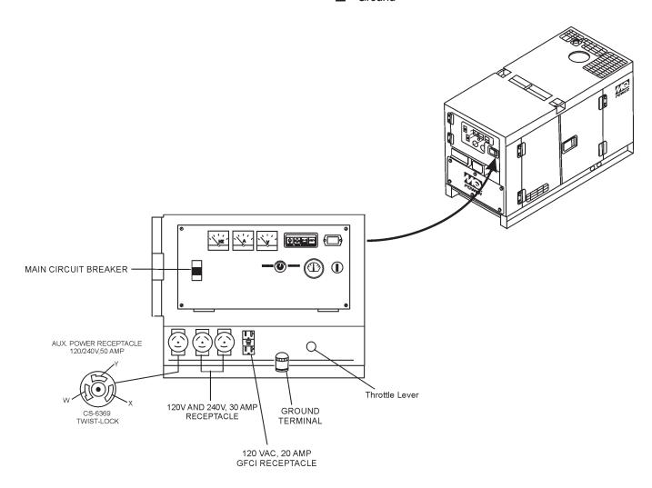
**Figure 5. Output Terminal Panel**
