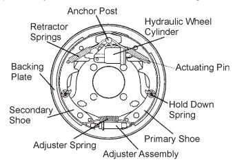
Figure 32. Hydraulic Brake Components
