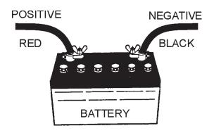
Figure 19. Battery Connections
