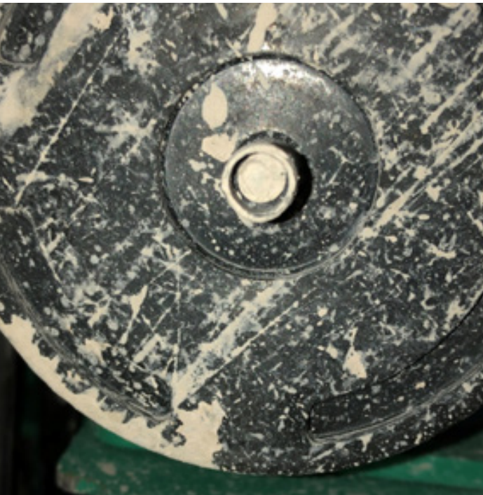
Shown is the charcoal canister that is part of the gasoline evaporative emission system. The lower air intake port in both photos are restricted or fully plugged with slurry. If the unit was switched from LPG fuel to gasoline, engine operation will be affected.
