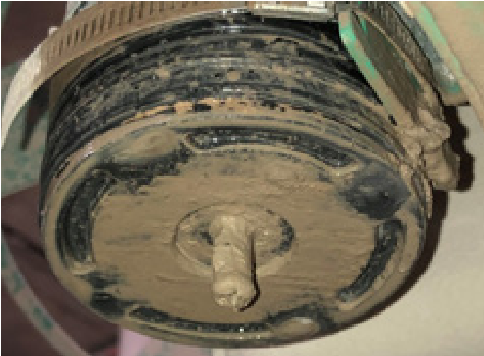
Shown is the charcoal canister that is part of the gasoline evaporative emission system. The lower air intake port in both photos are restricted or fully plugged with slurry. If the unit was switched from LPG fuel to gasoline, engine operation will be affected.
