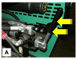
6. While observing the pressure gauge, squeeze the travel lever fully untill a deadhead pressure reading is obtained and let go of the travel lever, Ref. Figs. A & B, (Main Pump Minimum 2,250 PSI).
