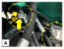
3. Start the engine and bring to full speed (3,600 RPM), while observing the pressure test gauge push the dump lever to full dump position and hold to obtain a deadhead pressure reading and return lever to center position, Ref. Figs. A & B, deadhead pressure reading should be (1,000 ~ 1,150 PSI).
