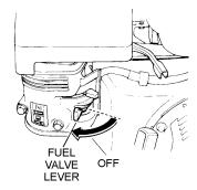
Figure 18. Fuel Valve Lever (OFF)
