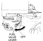
Figure 16. Fuel Valve Lever (OFF)
