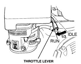
Figure 7. Throttle Lever (1/3 Start Position)
