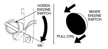
Figure 10. Engine ON/OFF Switches (ON Position)
