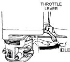
Figure 14. Throttle Lever (Idle)
