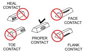
Figure 24. Gear Teeth Alignment
