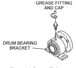
Figure 21. Grease Fittings (Dumping Mechanism)
