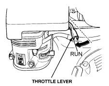
Figure 13. Throttle Lever (Run)
