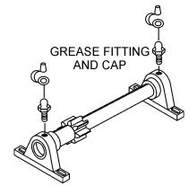
Figure 22. Grease Fittings (Countershaft)
