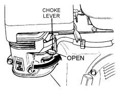
Figure 12. Choke Lever (Open)
