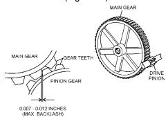
Figure 23. Drive Pinion and Main Gear (Backlash)
