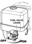
Figure 14. Fuel Shut-Off Lever
