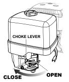
Figure 15. Choke Lever
