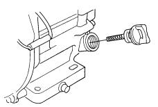
Figure 5. Engine Oil Dipstick (Removal)
