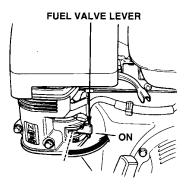
Figure 9. Fuel Shut-Off Lever
