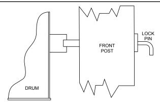
Figure 15. Drum Lock Pin (Side-View)
