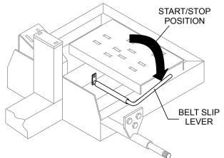
Figure 14. Belt Slip Lever (Start/Stop Position)
