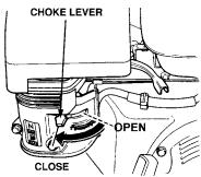
Figure 10. Choke Lever
