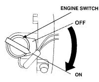
Figure 12. Engine On/Off Switch
