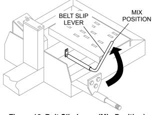
Figure 18. Belt Slip Lever (Mix Position)
