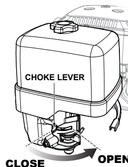
Figure 22. Engine Choke Lever (Open)
