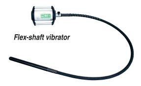
small pours that require a minimal amount of vibration (i.e. thin slabs, narrow walls, bases and small footings). In these cases, flex-shaft vibrators are usually sufficient. In pours with heavy rebar concentration, flex shafts can be used since small diameter heads (7/8" to 2") can avoid hang-ups in the rebar.
