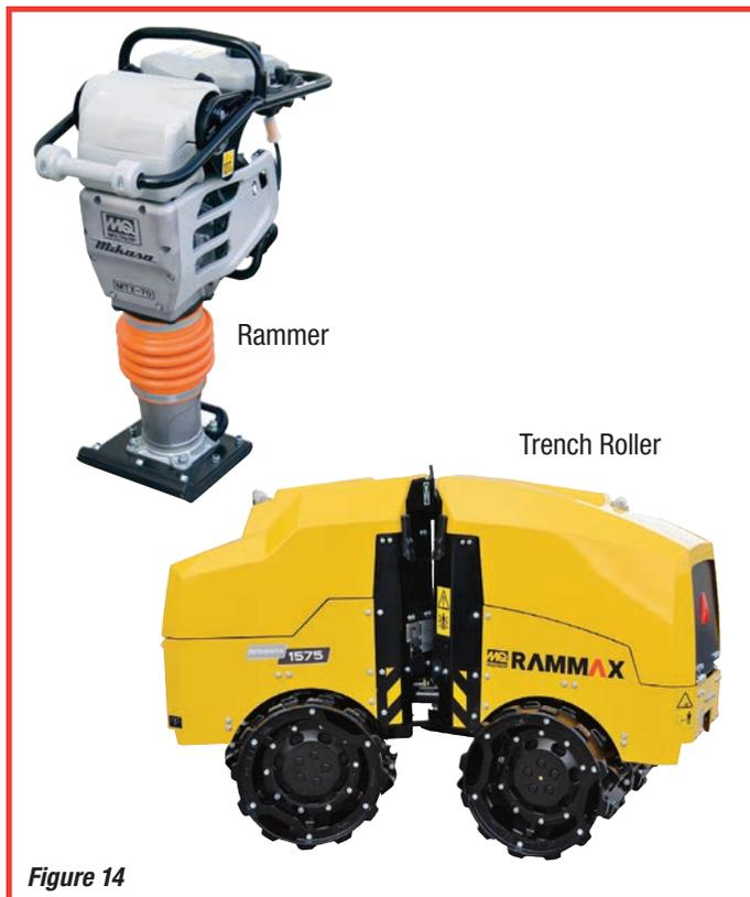
Reversible plates and smooth drum vibratory rollers are appropriate for production work. Granular soil particles respond to different frequencies (vibrations) depending on particle size. The smaller the particle, the higher the frequency necessary to move it. As you compact soils with larger particles, move up to larger equipment to obtain lower frequencies and higher compaction forces. [See Figure 15]
